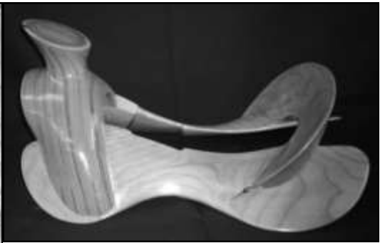
The finished tree, shellacked and ready for the rawhide cover and the final leather.
